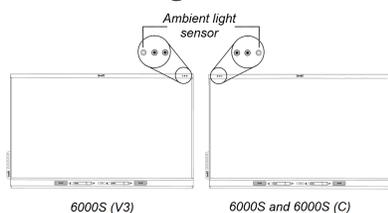
On SMART Board 6000S (V3) models, the ambient light sensor is located in the top-right corner of the display's frame. On the 6000S and 6000 (C) models, the sensor is in the top-left corner.
