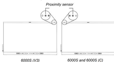
On SMART Board 6000S (V3) models, the proximity sensor is located in the top-right corner of the display's frame. On the 6000S and 6000S (C) models, the sensor is in the top-left corner.
