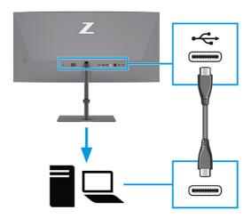
NOTE: The monitor's USB Type-C port provides network, data, video, and power delivery (up to 100 W).
