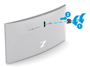
2. Align the Vesa adapter with the screw holes located on the rear of the monitor head (1), and then install the two screws to secure the adapter (2).
