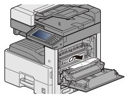
**3** Open the fuser cover (a) and remove any jammed paper.
