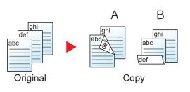
Produces two-sided copies from one-sided originals. In case of an odd number of originals, the back side of the last copy will be blank.
