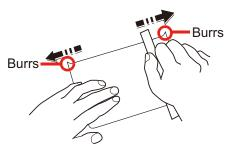
Before loading Hagaki (Cardstock), fan them and align the edges. Hagaki (Cardstock) should be fed from the MP tray with the print-side down or the cassette and the optional paper feeder with the print-side up. If the Hagaki (Cardstock) paper is curled, straighten it before loading. Printing onto curled Hagaki (Cardstock) may cause jams.
