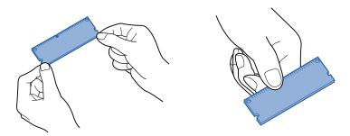
Electrostatic charge that builds up in the body through contact with clothing, carpeting, and other sources is a major enemy of chip memory. To protect memory from damage caused by electrostatic charge, touch a water tap or some metal object to discharge it from your body before loading the expansion memory. If possible, you should wear an antistatic wristband or take other anti-static measures.
