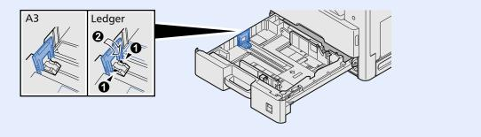
3 Adjust the position of the paper width guides located on the left and right sides of the cassette.
