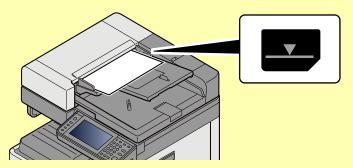
Ensure that loaded originals do not exceed the level indicator. Exceeding the maximum level may cause the originals to jam.
