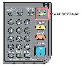
If print data is received during Sleep, the machine automatically wakes up and starts printing. Also when fax data arrives while the machine is in Sleep, the machine automatically wakes up and starts printing.
