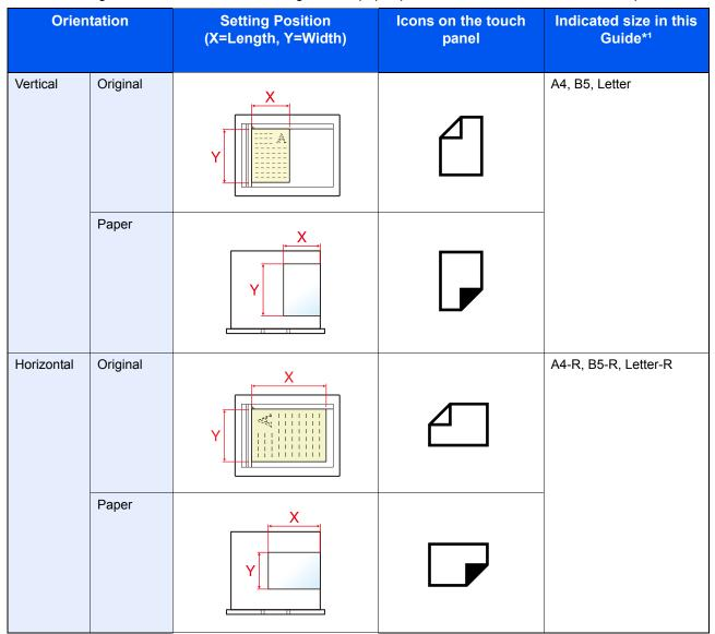
\*1 Original/paper sizes that can be used vary depending on the function and source tray. For details, refer to the following: →<u>Machine (12-21)</u>
