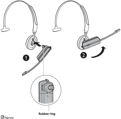
If you accidentally ripped off the rubber ring, use a spare rubber ring to replace it.
