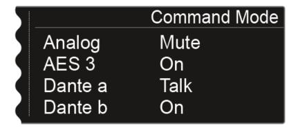
The **Analog** output signal is transmitted through the PA system for the audience. If the Command button on the transmitter is pressed, the signal on the PA system is muted. The signal is then activated on the **Dante a** channel on the Dante $^{\rm IM}$  network. The sound technician can then hear the signal for directional instruction.
