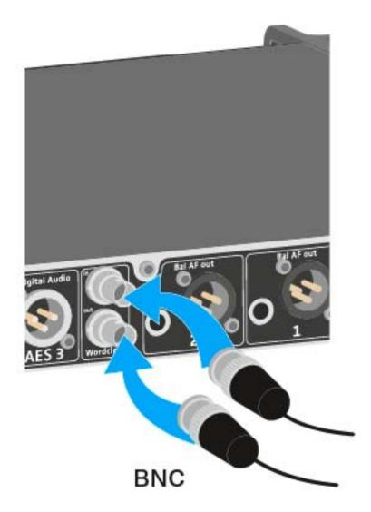
$\, \triangleright \,$  Use a coaxial BNC cable (75  $\Omega)$  to connect the external word clock to the  $\boldsymbol{Wordclock\ In}$  input.
