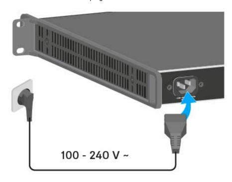
Once the EM 6000 is connected to the power supply, the **On/Off** button lights up dimmed. If the booster voltage for antennas is activated in the menu (see "System -> Booster Feed menu item"), it is active already before you switch on and after you switch off the EM 6000.
