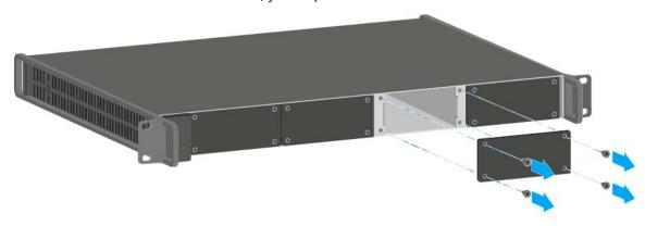
▶ Fully slide the charging module into the open charging slot as shown in the figure.
