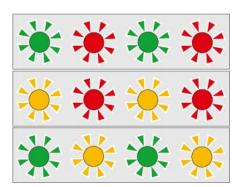
Flashing green/red >> rechargeable battery not inserted.
