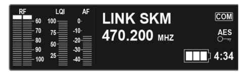
The first home screen that is displayed as the initial view after the device switches on contains the following status information.
