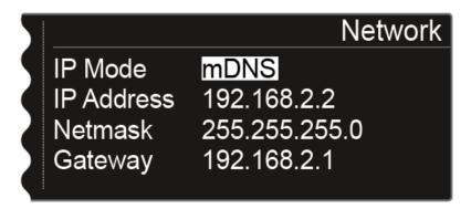
• IP Mode Manual: You can manually set the IP address, netmask, and gateway.
