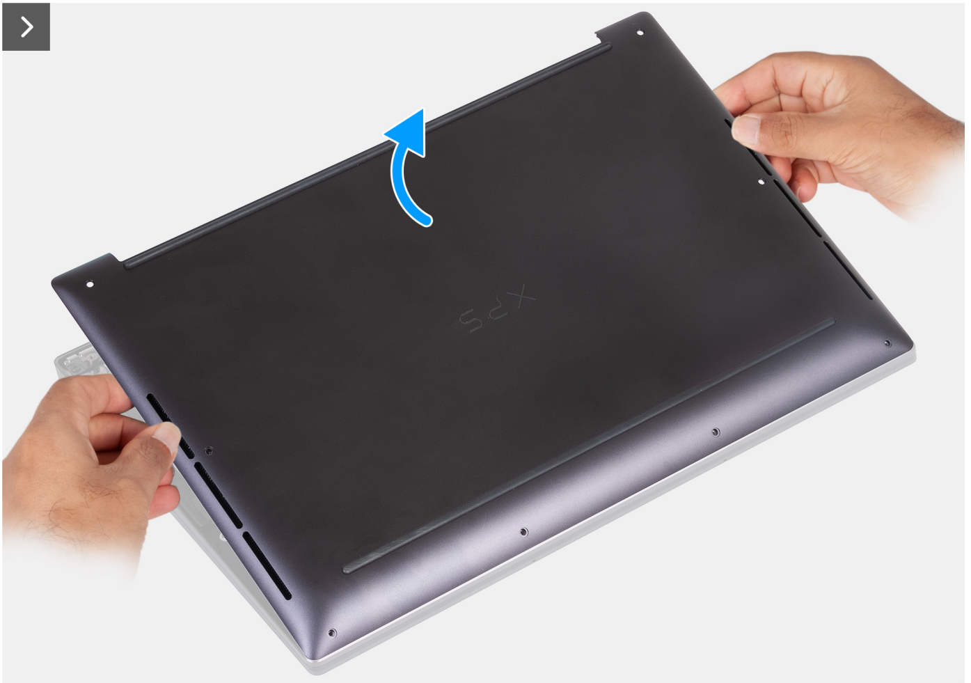
Figure 11. Lifting the base cover off the palm-rest assembly
