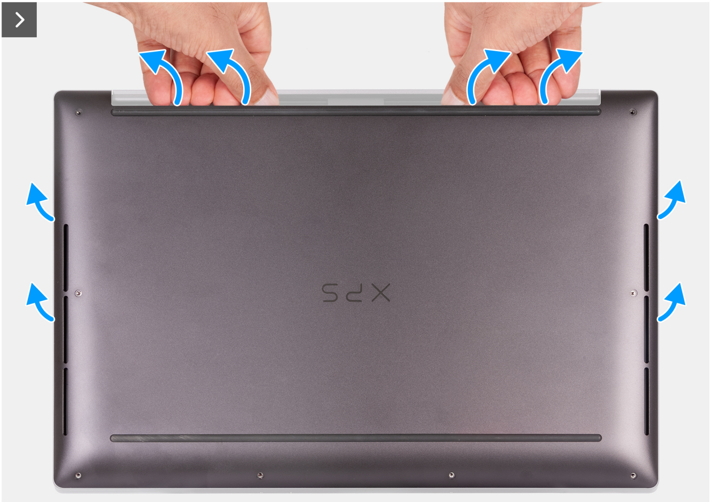
Figure 10. Using both thumbs to pry the base cover
