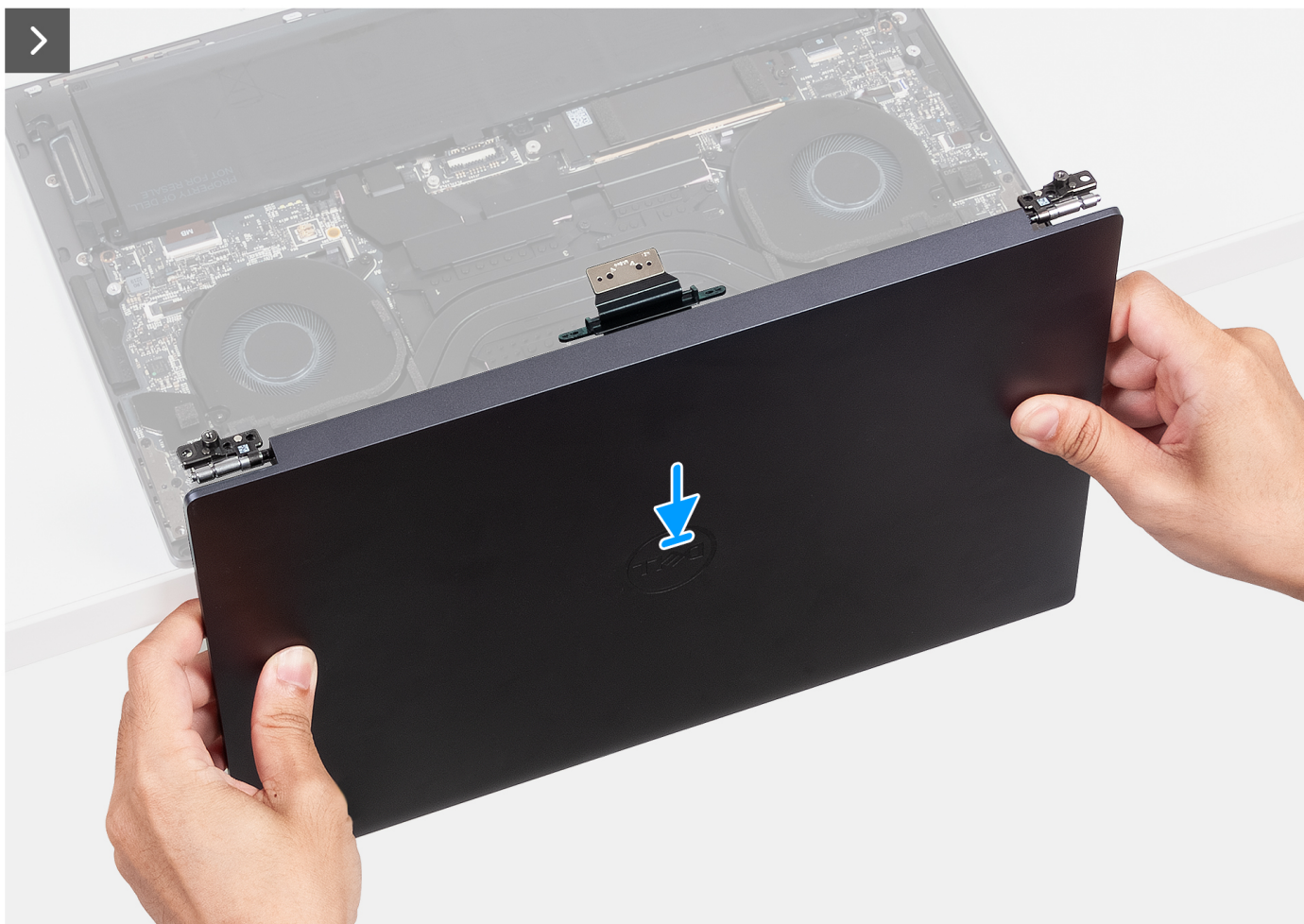
Figure 30. Installing the display assembly
