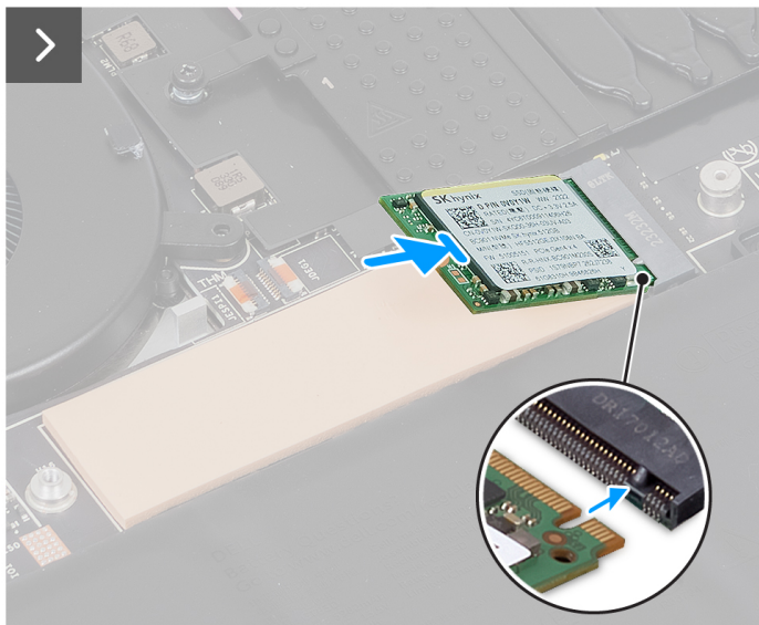
Figure 21. Installing the M.2 2230 solid-state drive
