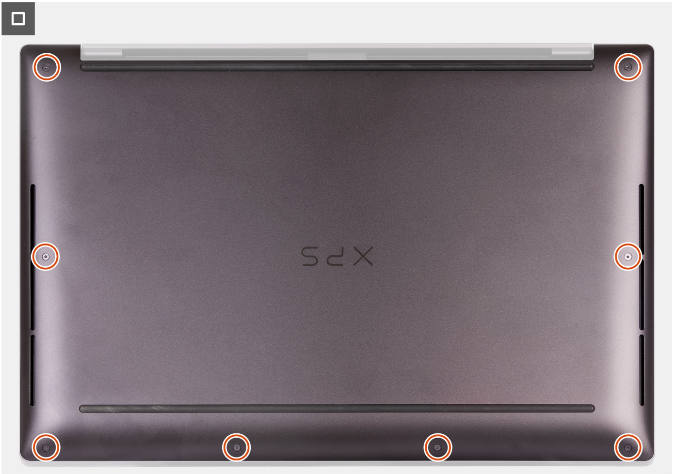
Figure 16. Tighten the eight screws that secure the base cover to the palm-rest assembly
