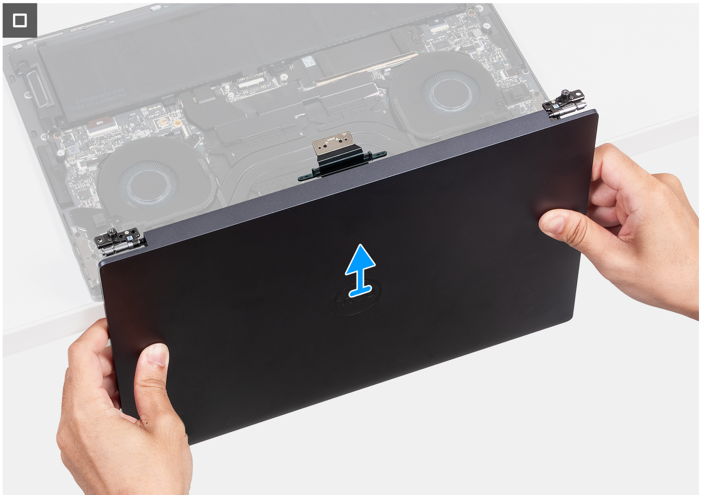
Figure 28. Removing the display assembly
