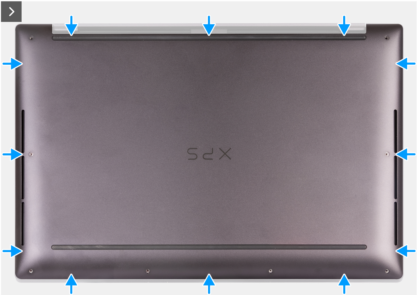
Figure 15. Snap the base cover into place on the palm-rest assembly
