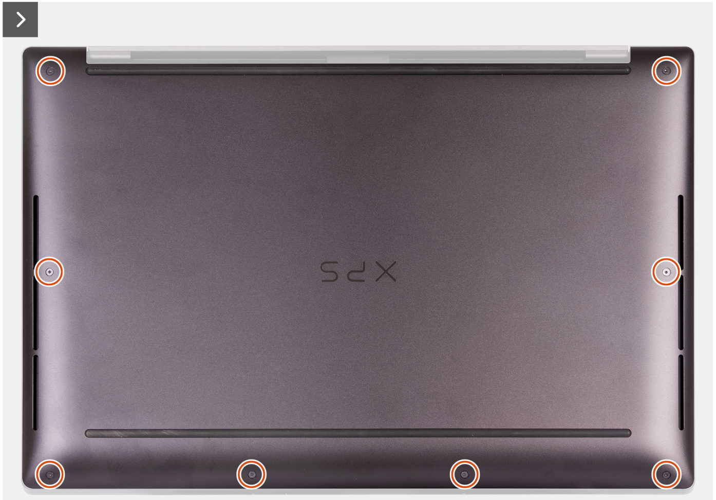
Figure 9. Removing the base cover
