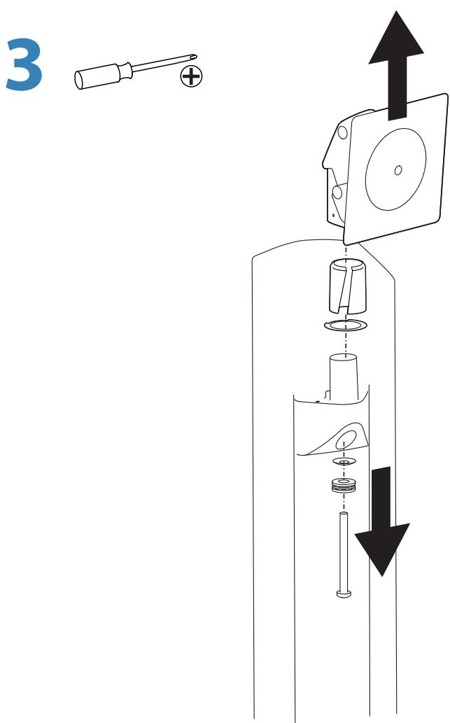
NOTE: Must seat fasteners fully to insure safety ground path.
