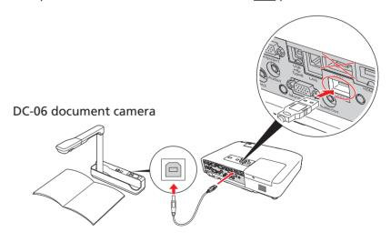
If you connect a digital camera or USB storage device, you can use the projector's EasyMP Slide Converter feature. See the *Network and PC Free Operation Guide* on your projector CD.
