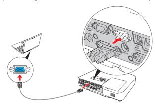
Connect one end to the projector's **Computer1** or **Computer2** port, and the other end to your computer's monitor port. If you are using a notebook, switch it to external display. You can also connect an audio cable.
