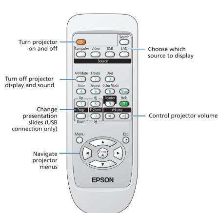
You can use the remote control to operate the projector. With the USB cable, you can use the remote as a wireless mouse. For more information on using the remote control, see your *User's Guide*.
