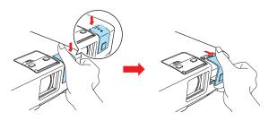
Insert the LAN module into the port and replace the cover.
