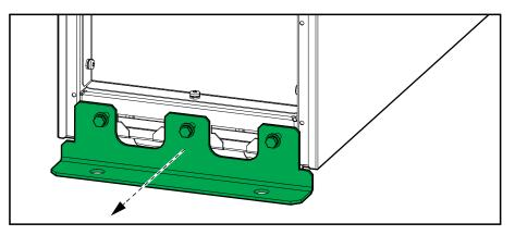
17. If the rear transportation bracket is available, install it on the rear of the UPS for increased stability.
