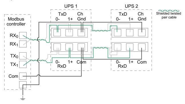
2. Install 150 Ohm termination resistors at each end of each bus if the buses are very long and operate at high data rates. Busses under 610 meters (2000 feet) at 9600 baud or under 305 meters (1000 feet) at 19.200 baud should not require termination resistors.
