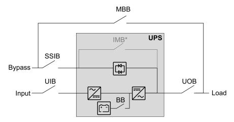
**NOTE:** The internal maintenance breaker IMB\* cannot be used in a system with an external maintenance bypass breaker MBB and the internal maintenance breaker IMB\* must be padlocked in the open position.
