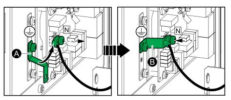
2. **Only for dual mains system**: Remove the indicated single mains jumper cables located behind the output/bypass terminals.
