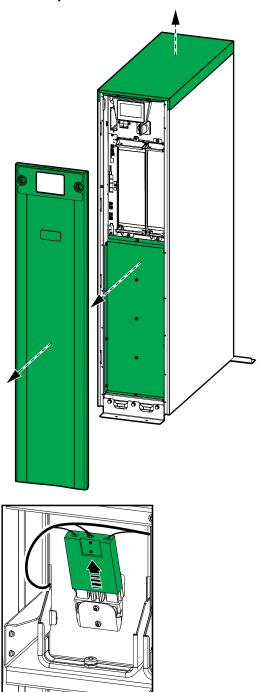
4. Remove the rear gland plates and the rear brush plates from the UPS. These are for signal cable routing.
