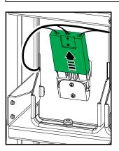
9. Remove the battery modules from the two upper rows. Leave the battery modules in the two bottom rows to increase weight stability.
