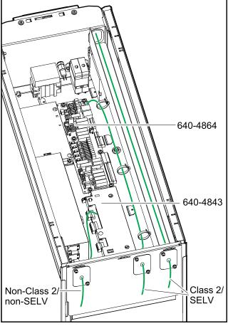
7. Route the Class 2/SELV signal cables through the middle rear brush/gland plate and into the UPS.
