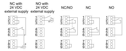
The EPO input supports 24 VDC.
