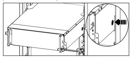
c. Install a filler plate (if available) in front of the empty power module slot.
