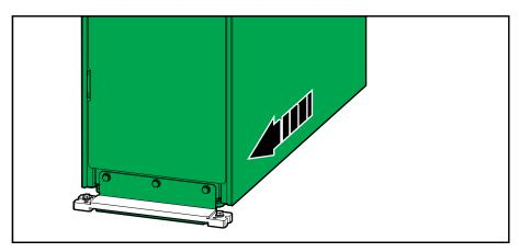
4. Lower the front and rear leveling feet on the UPS with a wrench until they connect with the floor. Use a bubble-leveler to check that the UPS is level.
