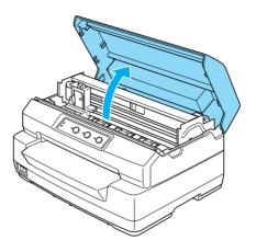
3. Push the release lever to move the upper mechanism forward. Make sure that you push the lever until it clicks.
