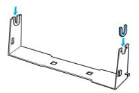
2. Place the base plate on the stand and fasten the two together with the plastic spacing clips. Make sure you orient the stand and base plate as shown below.
