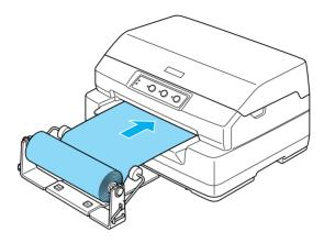
You are now ready to print. When you finish printing, advance the paper by holding the F2 button for a few seconds (in PR2 mode), or pressing the F1/EjeC1 button (in ESC/P or IBM PPDS mode). Then cut the roll paper where it comes out from the printer.
