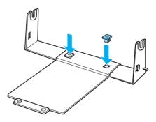
3. Hook the tension lever onto both ends of the stand as shown below. While pulling up on the tension lever, fit the wire ends of the tension lever into the holes in the stand. The roll paper holder is assembled.
