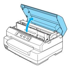
4. Push the release lever to move the upper mechanism forward. Make sure that you push the lever until it clicks.
