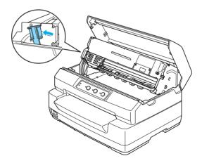
5. Slide the print head to the middle of the printer by hand.
