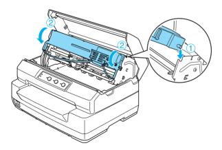
10. Hold both sides of the ribbon guide and pull it down until it is out of the cartridge.
