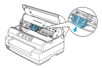
7. Hold both sides of the ribbon cartridge with both hands and rotate it on the plastic hooks. Then pull it up until it is out of the printer.
