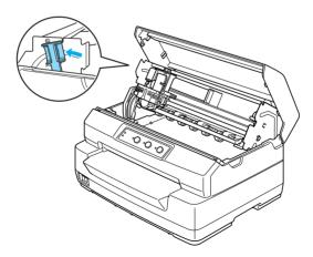
4. Slide the print head to the middle of the printer by hand.
