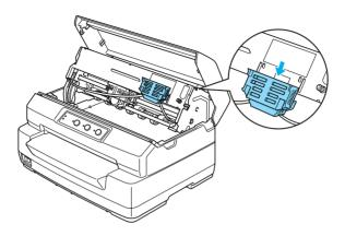
8. Put the ribbon guide at the bottom of the print head and push it up until it clicks into place.
