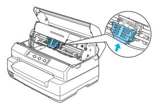
9. Turn the ribbon-tightening knob to help feed the ribbon into place.
