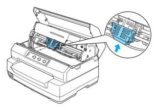
12. Turn the ribbon-tightening knob to help feed the ribbon into place.
