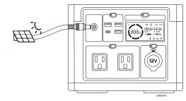
Connect the PSP100 solar panels to the DC input port of the Schneider OffGrid unit. Refer to solar panels installation guide for details.
