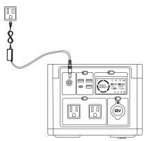
Connect the AC adapter to the wall outlet and the DC input port of the Schneider OffGrid unit.
