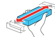
**Caution:** Do not touch the green chip on top of the cartridge. Doing so may prevent normal operation and printing.
