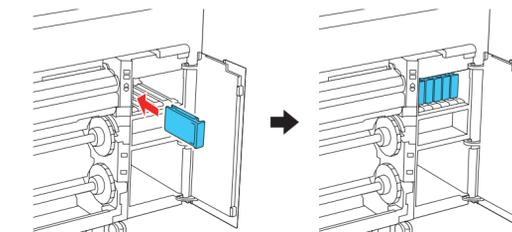
**Note:** Make sure all of the ink cartridges are properly inserted in the product; otherwise printing is not possible.
