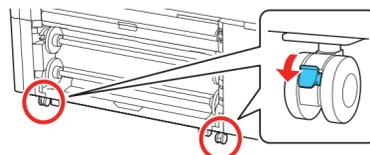
5 Secure the two adjustable feet on the back of the printer.
