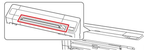
10 Remove the tape from the front of the printer and the paper catch basket.
