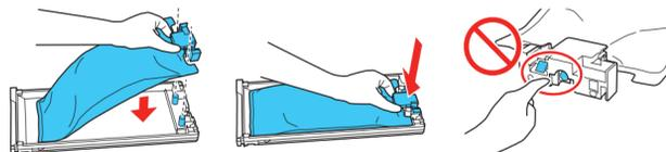
**Note:** Make sure the ink pack fits onto the pegs and is aligned with the top of the tray.
