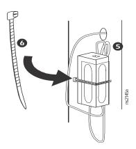
Plug the power cord into the top of the power supply.
