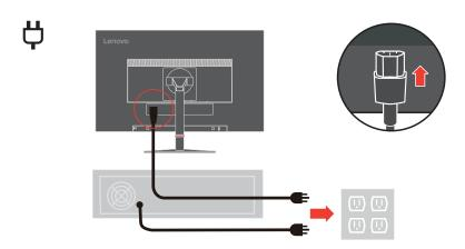
10. Connect the cables with cable clip.
