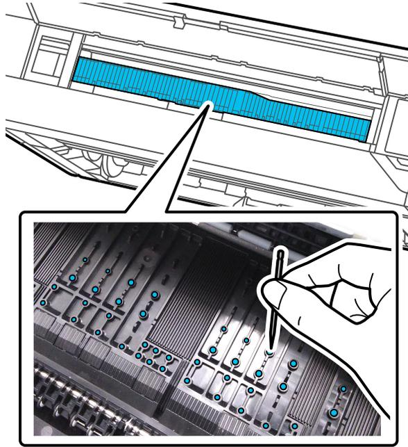
6. Use cotton swabs to remove any paper particles or dust around the outer edges of the borderless pads as shown.
