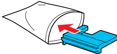
**Note:** Do not tilt the borderless maintenance box until the bag is firmly sealed, otherwise ink may leak.
