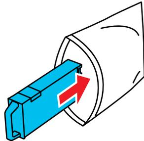
**Note:** Do not tilt the maintenance box until the bag is firmly sealed, otherwise ink may leak.
