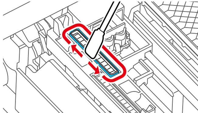
16. Hold the cleaning stick in a horizontal position and wipe the edges of the suction caps with the flat surface as shown.
