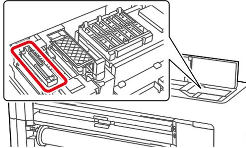
15. Hold the cleaning stick in a vertical position and wipe the outer areas of the suction caps as shown.
