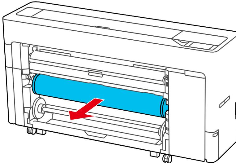
5. Remove the transparent paper stop from the spindle.
