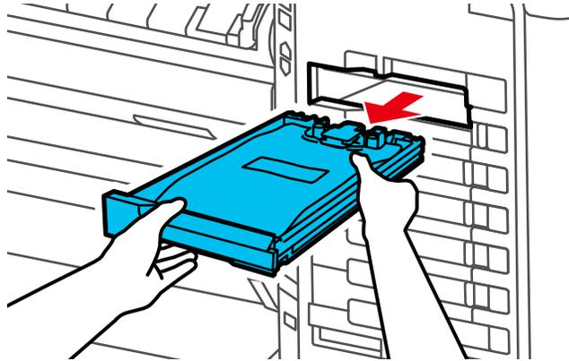
**Note:** Used ink packs may have ink around the ink supply port, so be careful not to get any ink on the surrounding area when removing the ink packs. Dispose of used ink packs carefully. Do not take the used ink pack apart or try to refill it.
