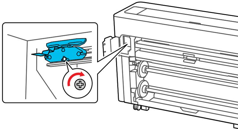
**Note:** Make sure the screw is tightened securely, otherwise the cut position may be slightly shifted or skewed.
