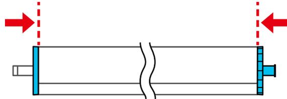
13. Place the spindle into the grooves on the Roll 2 unit with the black end of the spindle on the right, then push the Roll 2 unit in.
