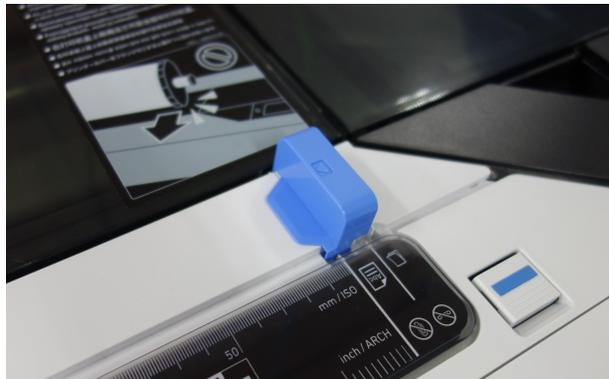
2. With the side to be scanned facing up, align the right edge of the original with the scanner edge guide.
