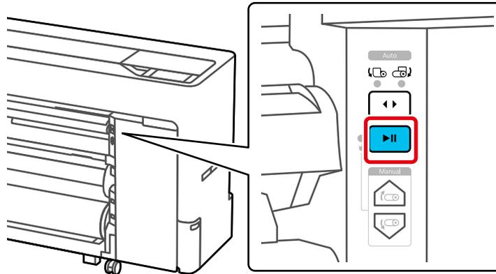
15. Use the take-up direction switch to select either printable side in (right) or printable side out (left), then press the pause/resume button again.
