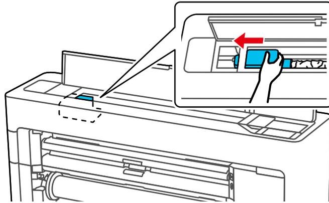
**Caution:** Do not touch the print head unless you are removing a paper jam. Touching the print head or the surrounding cables may cause a static shock and damage the printer.
