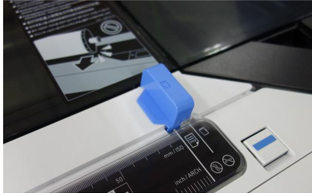
**Note:** Remove the scanner edge guide if you are using the carrier sheet.
