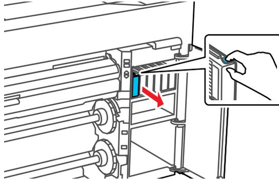
**Note:** Used ink cartridges may have ink around the ink supply port, so be careful not to get any ink on the surrounding area when removing the cartridges. Dispose of used cartridges carefully. Do not take the used cartridge apart or try to refill it.
