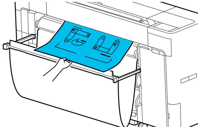
Printing starts when the original has been completely removed from the printer.
