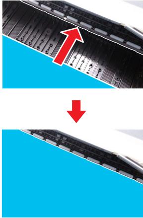
**When using cut sheets with a paper length shorter than 11.69 inches (297 mm):** Insert the paper past the alignment mark, making sure that it passes under the internal rollers.
