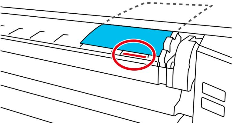
**Note:** Make sure the paper passes under the internal rollers as shown.
