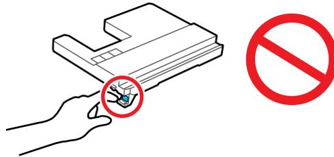
**Note:** Do not reuse a borderless maintenance box you have removed from the printer and exposed to air for a long period of time. The box will not absorb any more ink.
