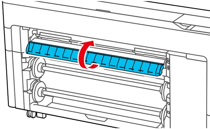
5. Pull up the lock lever on the roll paper holder.
