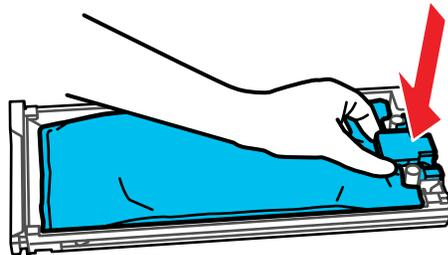
**Caution:** Make sure the ink pack fits onto the pegs and is aligned with the top of the tray.
