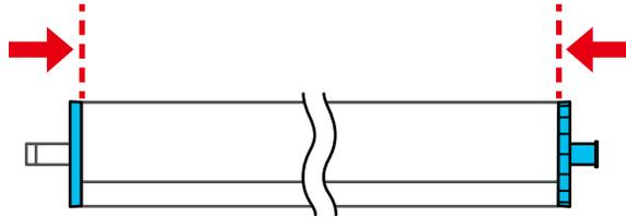
12. Place the spindle into the grooves on the printer with the black paper stop on the right.
