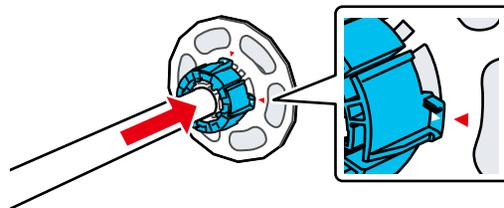
10. Insert the spindle into the roll core as shown.
