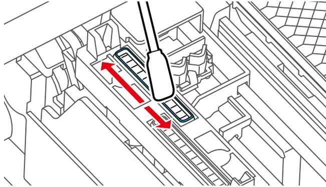
17. Hold the cleaning stick in a vertical position and wipe the guides shown here.
