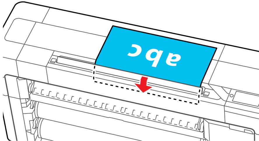
**Note:** When the automatic loading process begins, let go of the original and do not resist the loading process.
