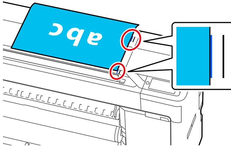
5. Support the original with both hands and insert the top edge into the scanner slot until it is automatically moved to the scanning position. You will hear a beep when loading is complete.
