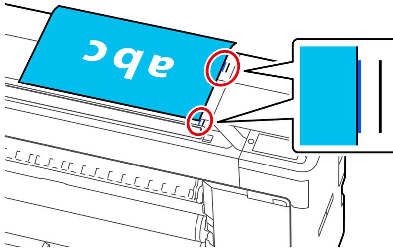
3. Support the original with both hands and insert the top edge into the scanner slot until it is automatically moved to the scanning position. You will hear a beep when loading is complete.
