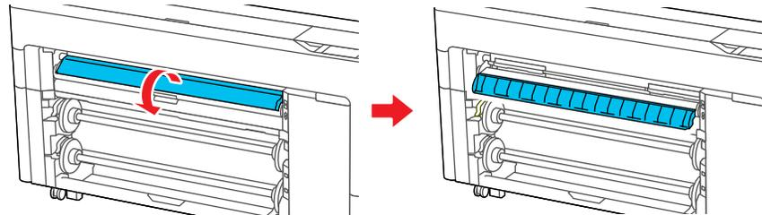
5. With the paper output flap extended, lift up the paper support lock lever, then move the paper support up to position **C** (the highest position) as shown.
