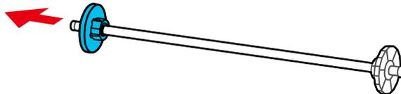
8. Remove the rim of the paper stop from the end of the spindle.
