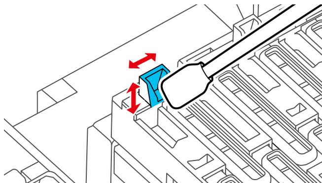
9. If there is any lint or dust in the drying prevention caps, remove it with the tip of the cleaning stick or a pair of tweezers.
