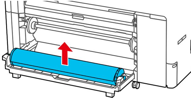
6. Remove the transparent paper stop from the spindle.
