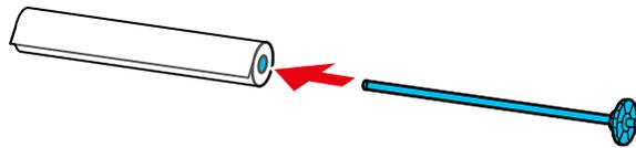
11. Attach the transparent paper stop to the spindle and press it in until there is no gap between the paper stop and the roll paper.
