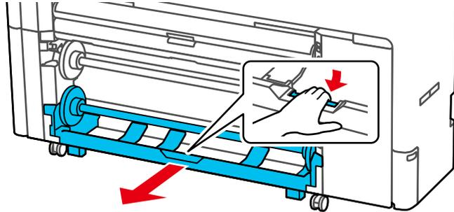
7. Remove the spindle.
