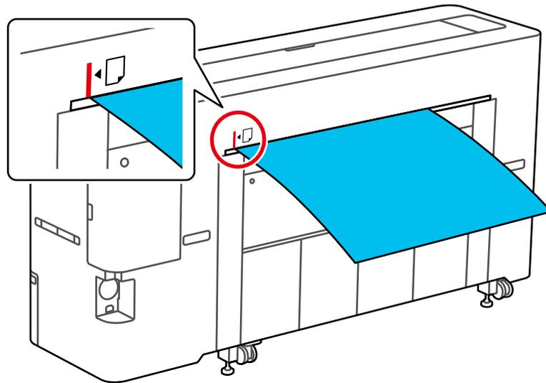
Feed the paper straight into the printer as shown.
