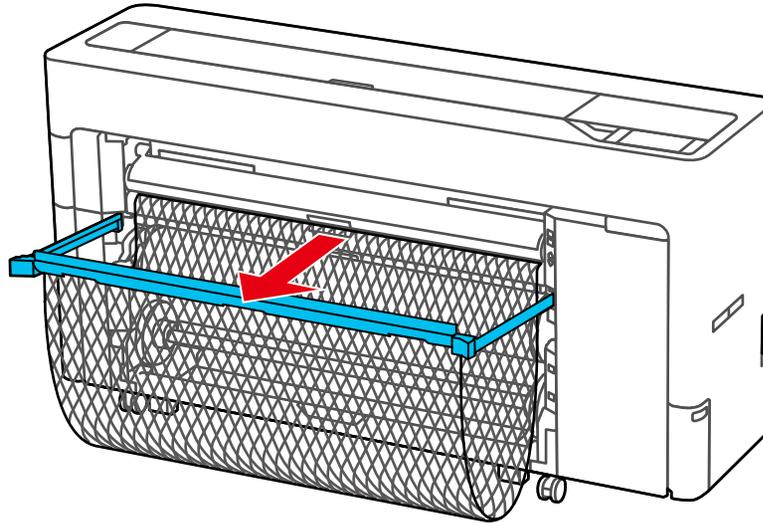
The basket can be used as a support to prevent the poster board from bending during printing.
