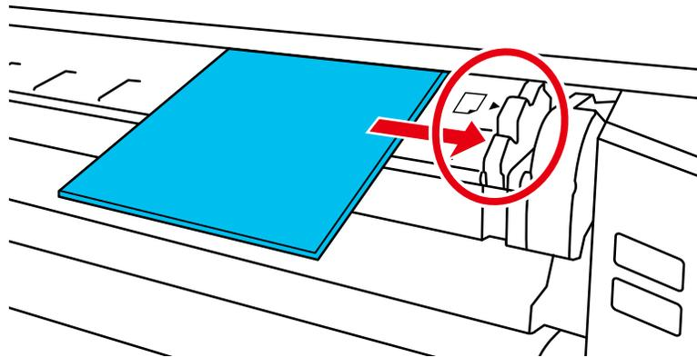
Insert the poster board straight into the printer until the trailing edge is above the loading mark on the roll paper cover (the top edge of the ruler).
