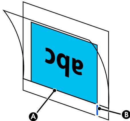
2. Insert the carrier sheet against the right side of the scanner slot.
