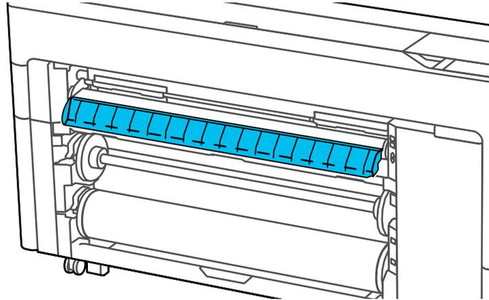
18. With the paper output flap extended, lift up the paper support lock lever to release the paper support, then set the paper support to position **B** (the middle position) as shown.
