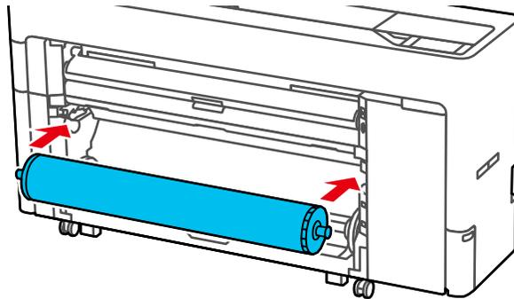
13. Push down the lock lever on the roll paper holder to lock it in place.
