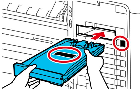
**Note:** The ink packs are keyed to fit into the correct color slot. If you cannot insert the ink tray all the way, do not force it. Make sure the ink pack color matches the color slot on the printer.
