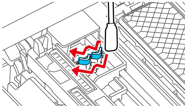
12. Wipe around the back of the wiper as shown.
