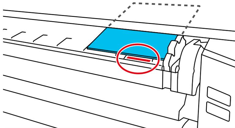
**Note:** Make sure the poster board passes under the internal rollers as shown.
