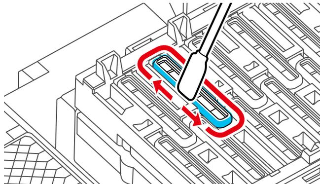
7. Hold the cleaning stick in a horizontal position and wipe the edges of the drying prevention caps with the flat surface as shown.
