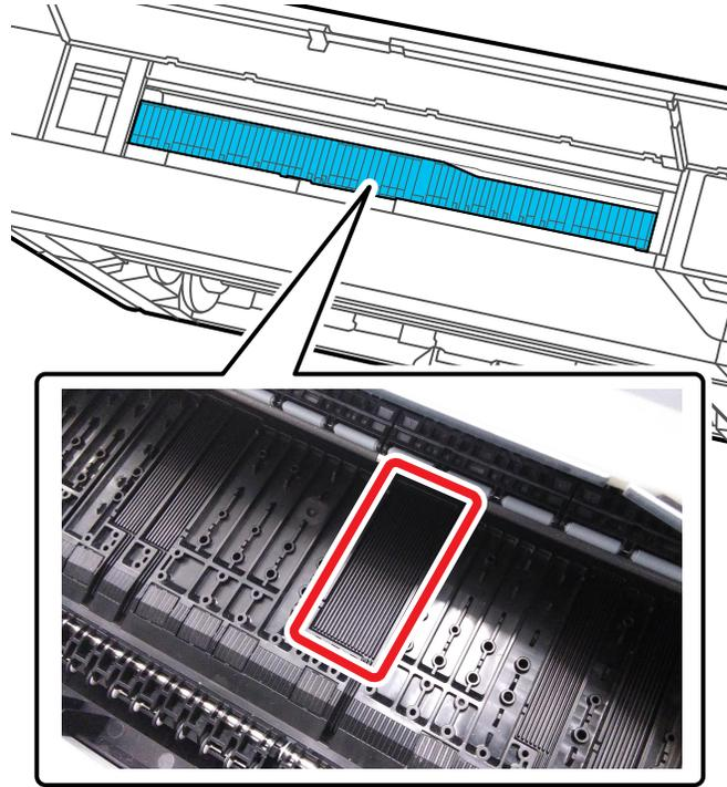
**Note:** For stubborn dirt, dampen a soft cloth with neutral detergent. Wring it out and clean the platen as shown above. Dry the platen with a soft, dry, lint-free cloth when you are finished.
