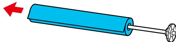
7. Re-attach the rim of the paper stop to the end of the spindle.
