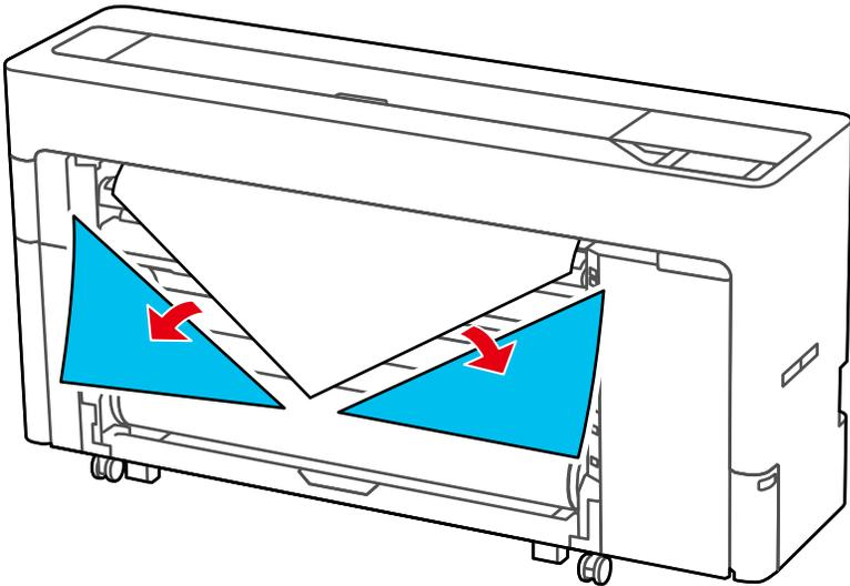
22. Confirm the take-up direction and tape the edge of the media to the center of the core as shown.
