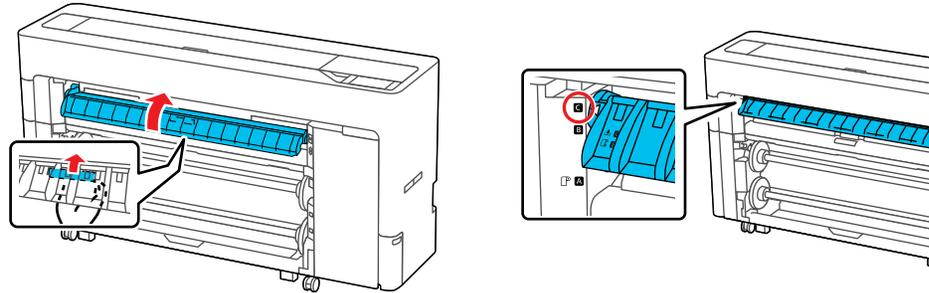
6. Pull out the borderless maintenance box carefully without tilting it.
