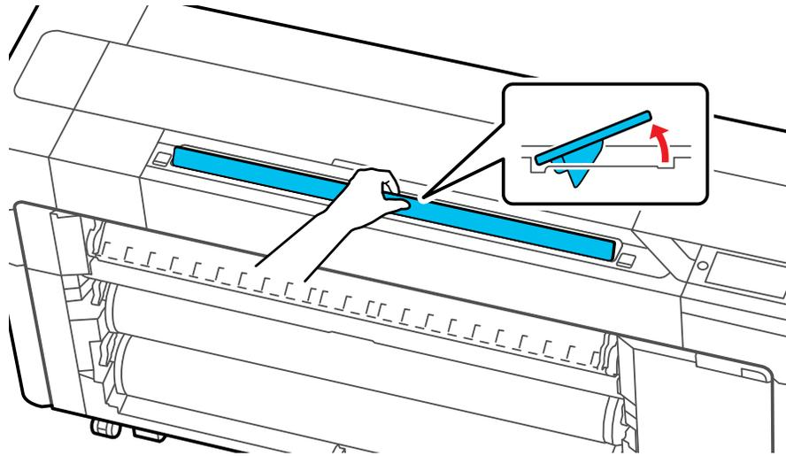
**Note:** Store the scanner edge guide when you open the scanner cover. If the document does not feed straight, install the scanner edge guide.
