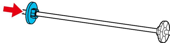
8. Place the spindle into the grooves on the printer with the black end of the spindle on the right.
