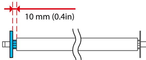
12. Place the spindle into the grooves on the printer with the black paper stop on the right.
