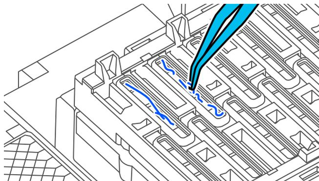
10. Use a new cleaning stick to wipe any dirt off of the wiper.
