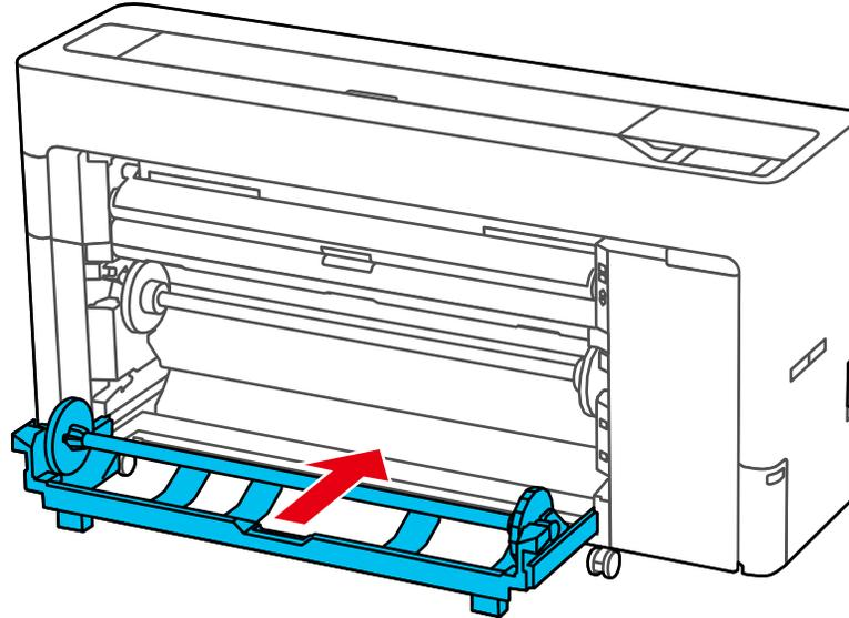
10. Push down the lock lever on the roll paper holder to lock it in place.
