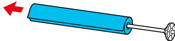
8. Reattach the transparent paper stop to the spindle.
