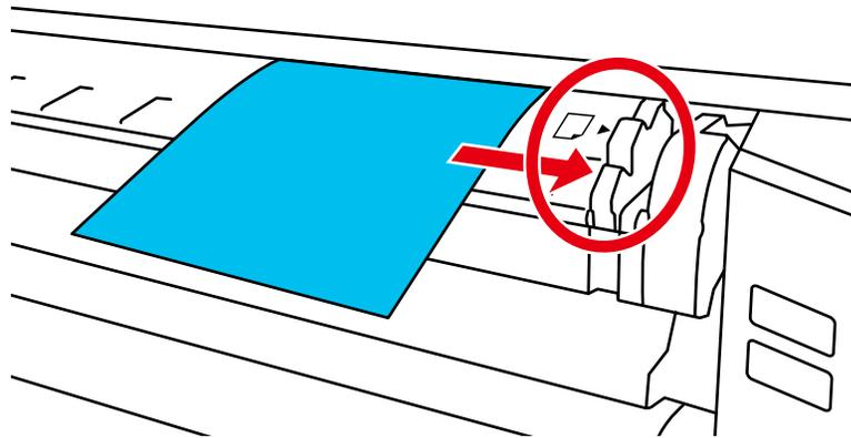
**When using cut sheets with a paper length of 11.69 inches (297 mm) or longer:** Insert the paper straight into the printer until the trailing edge is above the loading mark on the roll paper cover (the top edge of the ruler).
