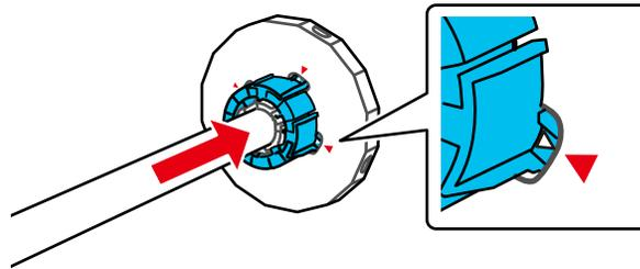
9. Insert the spindle into the roll paper core as shown, with the leading edge of the roll paper facing towards you. Push the fixed paper stop against the roll paper until there is no gap between the paper stop and the roll paper.
