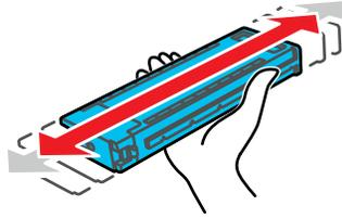
6. Insert the new cartridge into the corresponding ink slot and push it in firmly.
