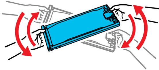
7. Match the color on the ink pack label with the color slot on the printer, then insert the ink tray into the slot and push it in firmly.
