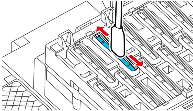
6. Hold the cleaning stick in a vertical position and wipe the outer areas of the drying prevention caps as shown.
