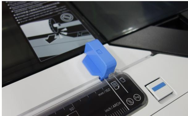
4. With the side to be scanned facing up, align the right edge of the original as shown.
