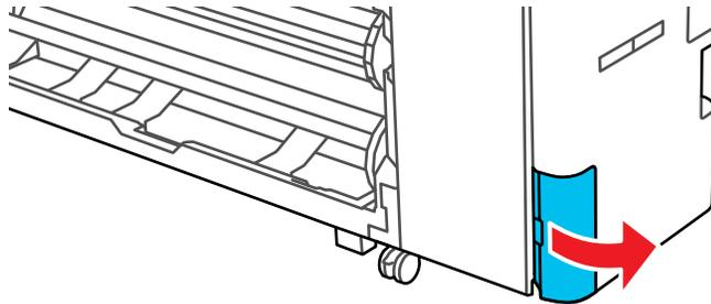
4. Use the handle on the maintenance box to carefully pull it out of the product without tilting the box.
