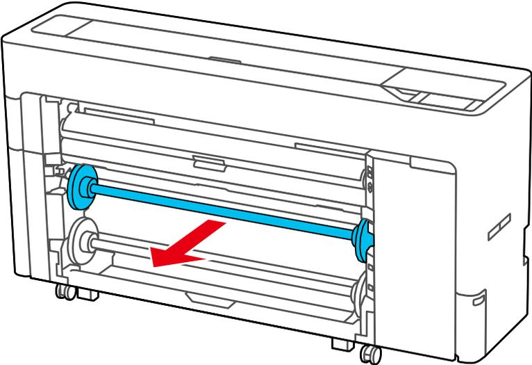
7. Remove the transparent paper stop from the spindle.
