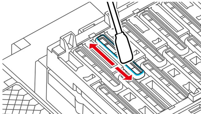
8. Hold the cleaning stick in a vertical position and wipe the guides as shown.
