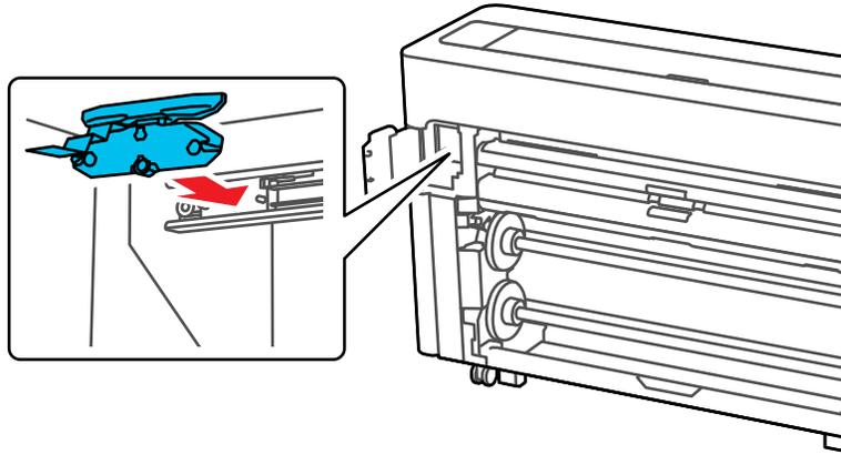
7. Tighten the cutter screw securely.
