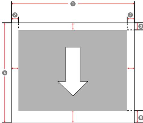
**Note:** Margins may change depending on the **Top Margin** setting that you select. If you select **Save Roll Paper** as the Roll Paper Option on the printer driver's Advanced tab, the top and bottom margins of the paper are set to 0 mm. The margins listed below are the standard settings. When printing with the left and right borderless setting, the left and right margins are set to 0 mm. When printing with the borderless on all sides setting, all margins are set to 0 mm.
