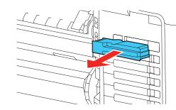
Insert the ink pack into the tray with the color label facing up and push 3 it down as shown.
