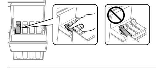
6. When you have finished refilling the ink, remove the ink bottle, and then close the ink tank cap securely.
