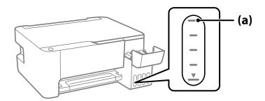
5. Align the top of the ink bottle with the filling port, and then insert it straight into the port to fill ink until it stops automatically at the upper line.
