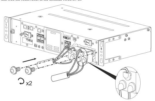
**Note:** The strain relief should be installed based on the routing of the input and output wires. The wires can be routed up or down from the strain relief.
