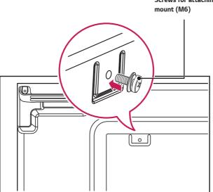
Screws for attaching the VESA wall mount (M6)
