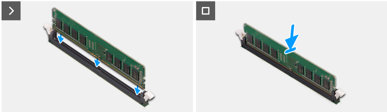
Figure 24. Installing the memory module
