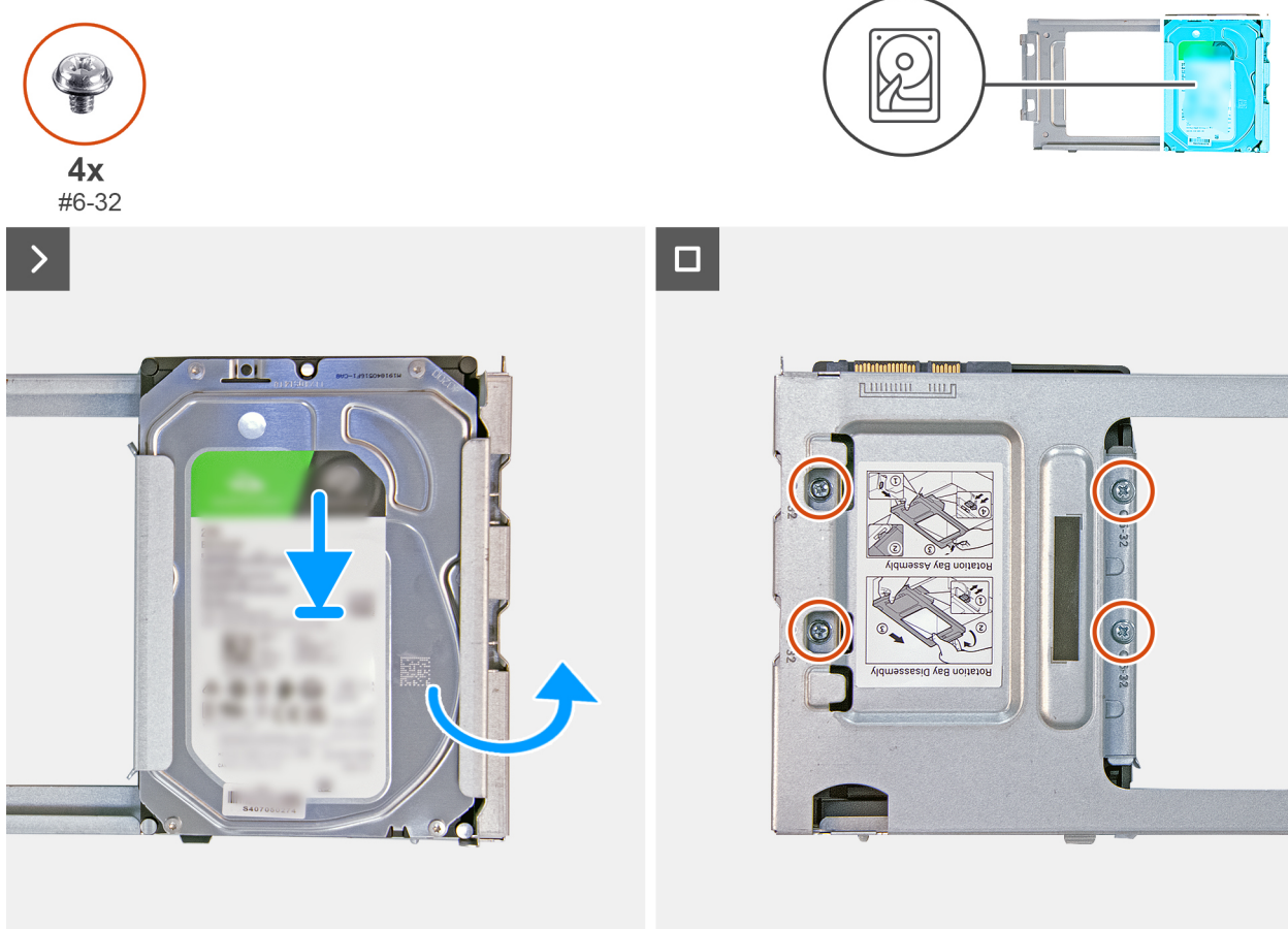
Figure 22. Installing the hard drive
