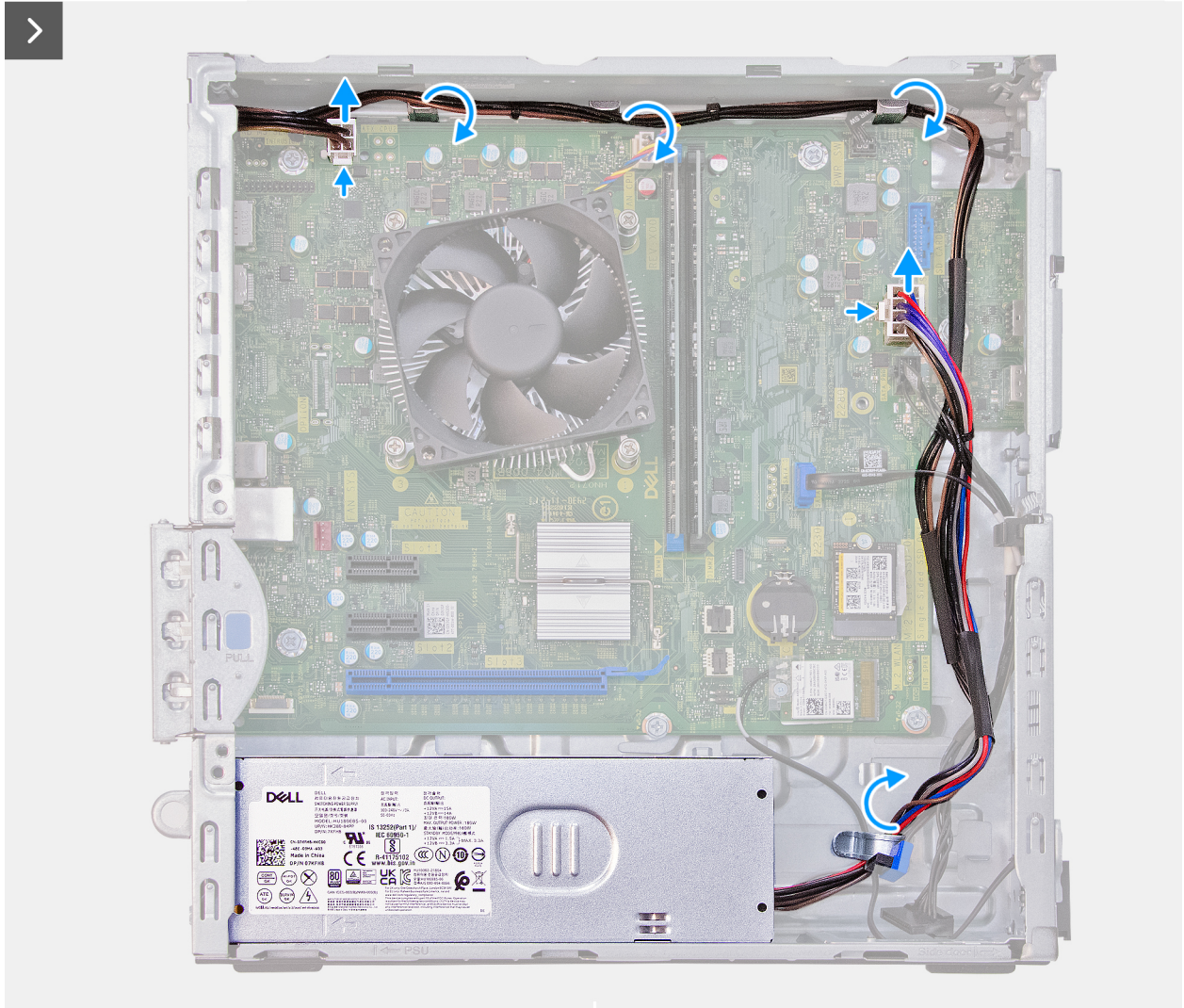
Figure 33. Removing the power-supply unit
