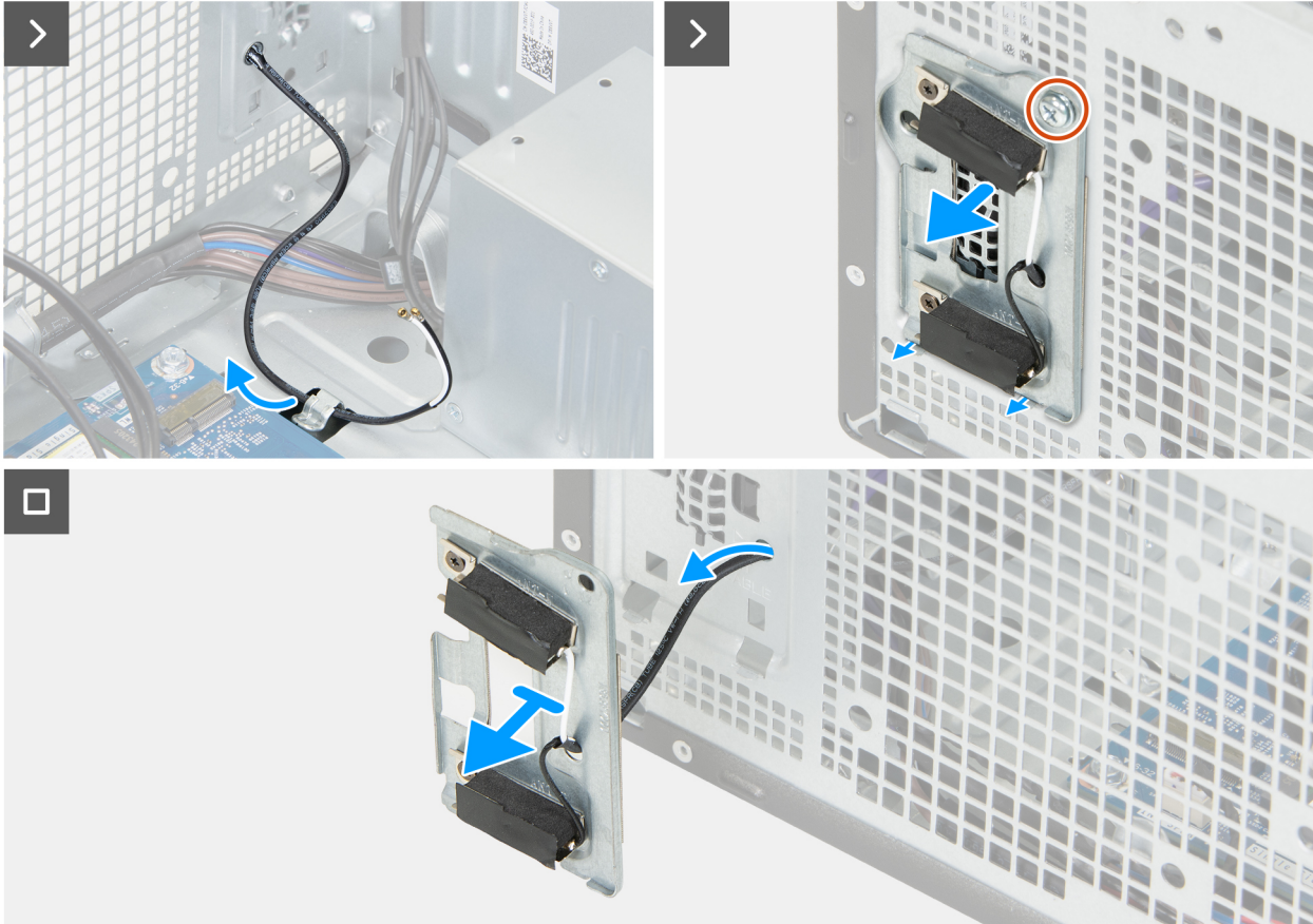
Figure 31. Removing the antenna module
