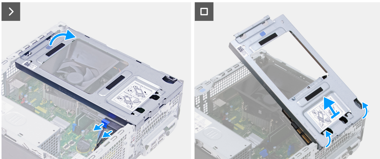
Figure 18. Removing the drive bay
