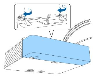
To remove the cover, loosen both screws and pull the cover off of the projector.
