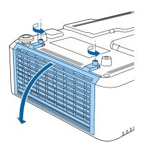
3. Pull the air filter out of the projector.
