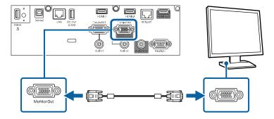
**Note:** You can only output analog RGB signals from the Computer1 port to an external monitor. You cannot output signals from other ports.
