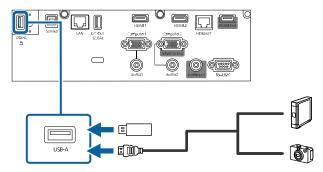
3. If you connected a USB cable, connect the other end to the USB device as necessary.
