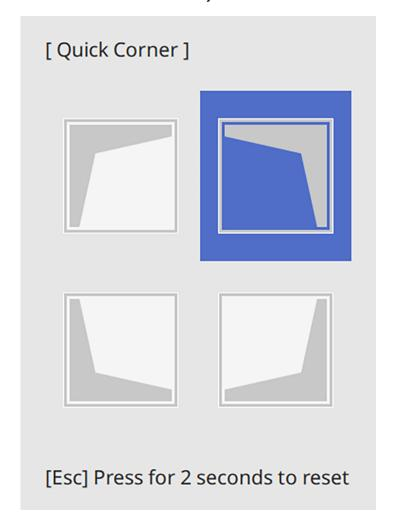
**Note:** To reset your adjustments, press and hold the **Esc** button for at least 2 seconds to display a reset screen. Then select **Yes**.
