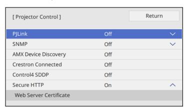
5. Set the **Crestron Connected** setting to **On** to allow the projector to be detected.
