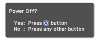
The projector beeps twice, the laser turns off, and the Status light turns off.
