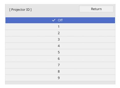
4. Press the arrow buttons on the remote control to select the identification number you want to use for the projector. Then press **Lenter**.
