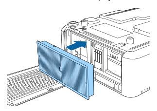
9. Replace the air filter cover and tighten the screws as shown.
