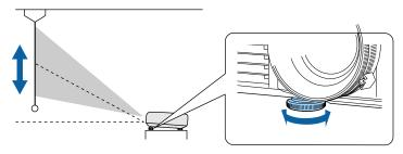
3. If the image is tilted, rotate the rear feet to adjust their height.
