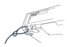
**Note:** Do not pass drop-prevention cables through the security cable attachment point when mounting the projector on a wall or ceiling.
