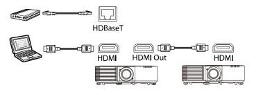
**Note:** If you are connecting three or more projectors, connect the projectors in a chain as shown.
