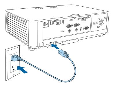
2. Plug the power cord into an electrical outlet.
