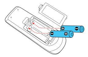
**Warning:** Make sure the batteries are inserted in the correct positions. If the batteries are not inserted correctly, they could explode or leak, causing a fire, injury, or damage to the product.
