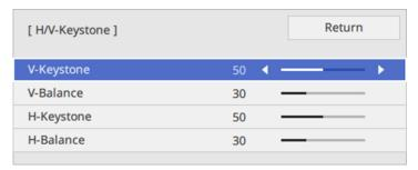
6. Use the arrow buttons on the projector or the remote control to select between vertical and horizontal keystone or balance correction and to adjust the image shape as necessary.
