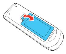
2. Insert the batteries with the + and – ends facing as shown.
