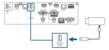
**Note:** To keep supplying power to the optional streaming media player when the projector is not projecting images, select **Always On** as the **USB Power** setting in the projector's Operation menu.
