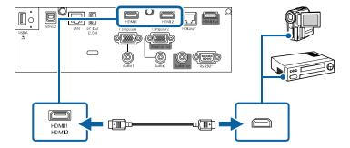
**Note:** If you have problems hearing audio through the HDMI connection, you can use one of the projector's audio ports instead to play sound. Connect one end of an optional 3.5 mm stereo mini-jack
