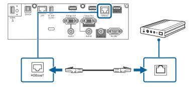
**Note:** See the documentation that came with the HDBaseT transmitter for instructions on connecting it to your video device or computer.
