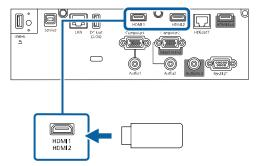
2. If necessary, connect the streaming media player's USB power supply cable to the **DC Out (2.0A)** port. Connect the other end of the cable to the USB port on the streaming media player.
