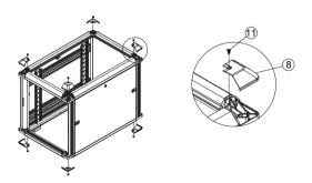
3. (Optional) Install the Casters (20) / Brake Casters (21) on the bottom of the rack using the M6-10mm Tapping Screws (22). Then thread the Leveling Feet (23) into the pre-threaded holes.
