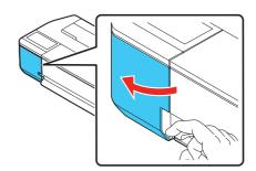
A Remove the tape and the protective piece.
