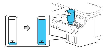
Note: If ink does not flow from the bottle, lift and reinsert the bottle.
