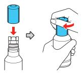
**Note:** Do not leave the ink bottle inserted; otherwise the bottle may be damaged or ink may leak.
