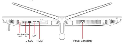
3.A. Please do not connect the DisplayPort out on the monitor to the DisplayPort or mini DP connector on the computer. DisplayPort out is used for daisy chain connection (Explained in section C)
