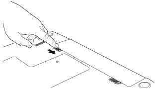
(Sample Illustration) Locking the battery release lock
