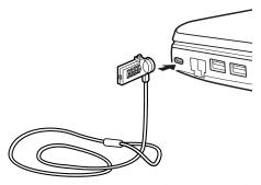
(Sample Illustration) Attaching security lock cable
