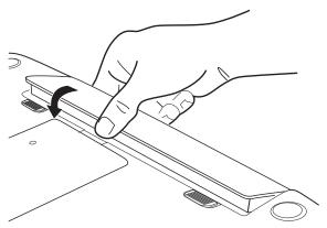
(Sample Illustration) Inserting the battery
