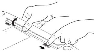
(Sample Illustration) Removing the battery
