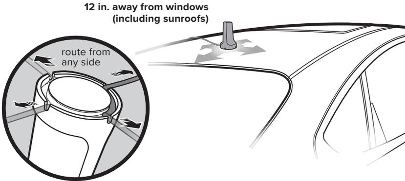
NOTE: For aluminum roofs, an **adhesive disk** is included to mount the outside antenna (do not use if outside antenna will magnetize to the top of your vehicle).
