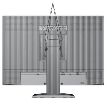
Step 3. Four screws attaching the base
