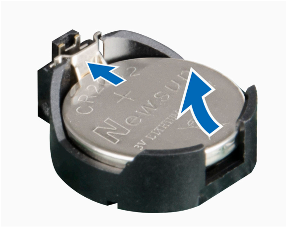
Figure 48. Removing the system battery
