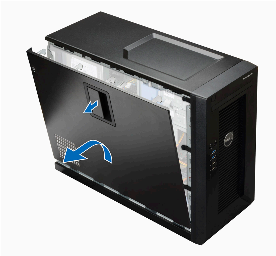
Figure 7. Removing the system cover
