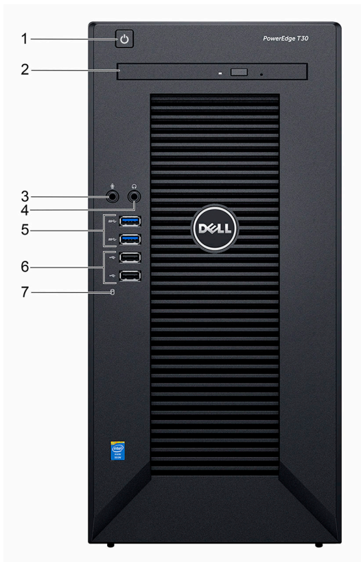
Figure 2. Front panel features and indicators
