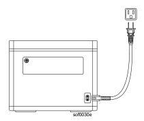
Connect the AC charging cable to the wall outlet and the input port of the Schneider OffGrid unit.
