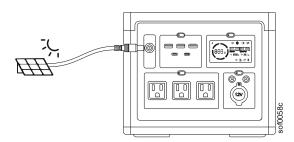
Connect the PSP100 or PSP200 solar panels to the DC input port of the Schneider OffGrid unit. Refer to solar panels installation guide for details.
