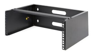
The 4U 13.78in. (35cm) deep wall-mounting bracket for patch panels and network equipment, delivers a sturdy and dependable equipment storage option, allowing you to wall mount data/IT equipment up to ta total of 44lbs. (20kg). It's the perfect solution for areas where space is at a premium like small office/home office environments or spaces with limited server room because it doesn't take up any floor space.
