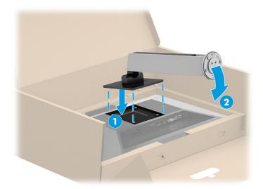
**3.** With the monitor still placed facedown inside the box, insert the base into the bottom of the monitor stand (1), and then swivel the base counterclockwise to lock it in place (2). Confirm that the arrow on
