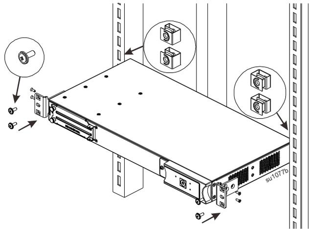
3 Secure clip nuts to the rack, and attach brackets with provided screws.
