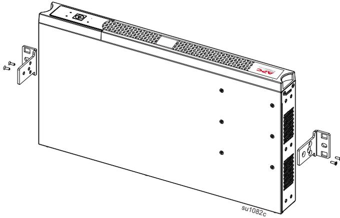
2 **Note:** Whenever possible, attach two screws into wall studs. If stud mounting is not possible, use an expandable wall anchor. Hardware is not included; .25" x 2" lag bolts are recommended. Mount the UPS in either of the displayed positions.
