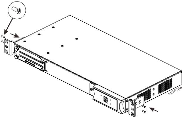
2 *Two-post rack-mounting:* Utilize the bracket holes that are offset 6.25".
