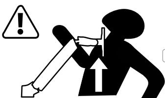
**[EN]** WARNING! Stored Energy Hazard: The Riser mechanism is under tension and will move up rapidly, on its own, as soon as attached equipment is removed. For this reason, DO NOT remove equipment unless the Riser has been moved to the highest position! Failure to follow this instruction may result in serious personal injury and/or equipment damage!
