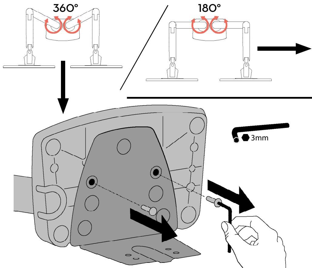
How to replace rotation stop screws (Arms must be straight up)
