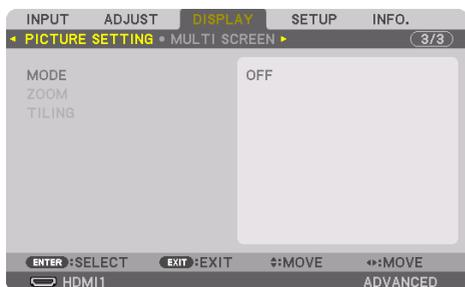
This sets the division conditions for reducing or enlarging the image area and displaying it in the desired position or for projecting using a combination of several projectors.
