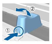
When installing, hook them into the printer cover, and press the button.
