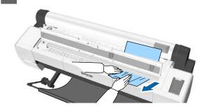
After removing the paper, reload the paper and restart printing.
