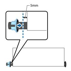
When you installed the tensioner, press the button. ►
