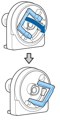
Attach an adapter to each end of the roll.
