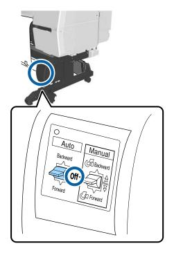
Hold down the Manual button in the taking-up direction to wind the paper around the roll core twice.
