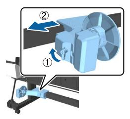
Insert flange R into the roll core.
