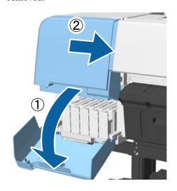
Attach the screws, and then close the cartridge cover.
