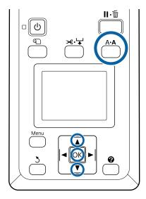
Confirm that the printer is ready and press the A-A button.
