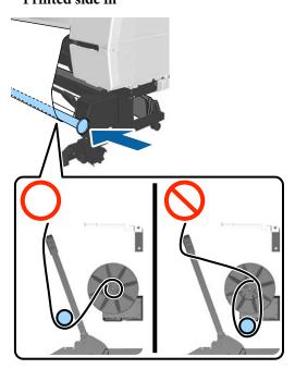
Align flange R for the tensioner with the right end of the paper.
