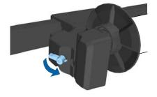
Make sure that the roll core is fixed in place and cannot move around.
