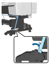
☐ The sensor on the stand is lowered, and the casters on the front are parallel to the stand
