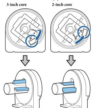
Lift up the adapter lock lever to release the lock on each of the two roll paper adapters.
