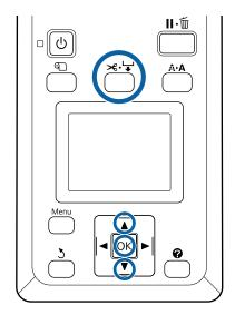
Press the ★ button. While viewing the inside of the printer through the window, hold down the ▼ button until the cutting position reaches the mark on the label.
