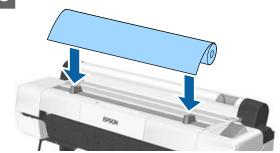
Move the size switch levers of the two supplied roll paper adapters in accordance with the roll-core size of the roll paper to be loaded.
