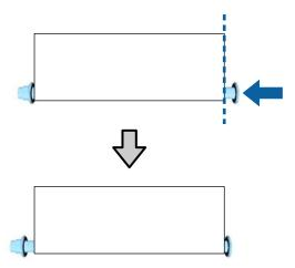
Move flange L for the tensioner to create a gap of approximately 5 mm from the left end of the paper.
