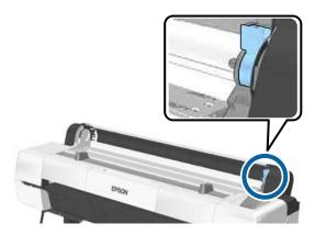
Remove the roll paper from the roll stand, slide the roll paper right until it contacts the adapter guide, and then slide the roll slowly inside.
