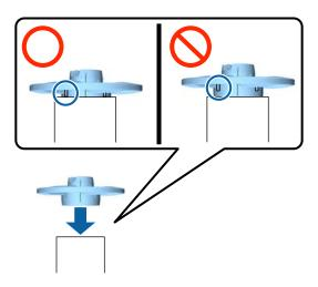
Install the roll core with the flange attached into the unit on the right of the printer.
