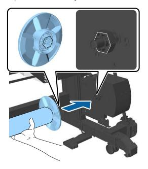
Move the unit on the left of the printer, and insert the flange in the end of the roll core.
