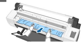
Unlock the roll paper lock lever, and then rewind the paper.
