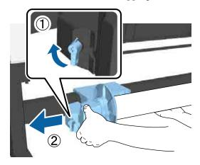
Remove the roll core from the auto take-up reel unit.
