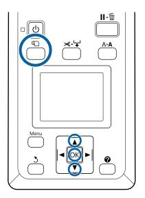
Press the ⑤ button on the control panel./Use the ▼/▲ buttons to select **Use Take-up Unit**, and then press the **OK** button.
