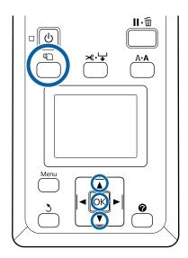
Confirm that the printer is ready and press the D button.
