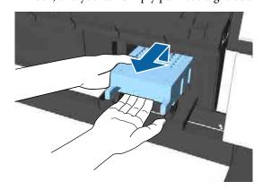
Place the used maintenance box in the clear bag included with your new maintenance box, and make sure that the zipper is closed tight.
