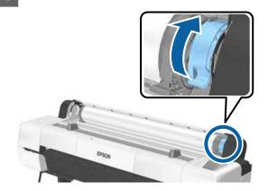
Remove the roll paper from the adapter holders, and place it in the roll rests.
