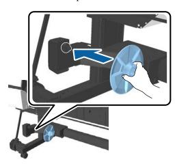
Unlock the unit on which flange L is installed, and then move it until it is to the left of the roll core width to install.
