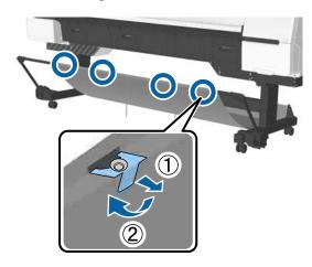
2 Loosely roll up the removed cloth with the top surface of the cloth inside, and insert the loop into the clamps hanging down from the printer.
