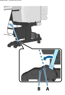
Press the ▶ button after moving the support bar.
