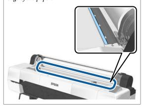
While lightly pressing the roll paper, lower the lock lever, and press the OK button.
