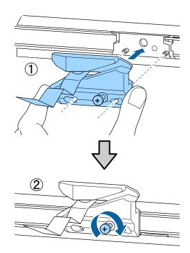
After replacing the cutter, press the **OK** button.
