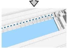
Align the right and leading edges of the paper with the lines on the poster board support as shown in (2).
