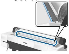
☐ For Epson Color Calibration Utility color charts, insert the page from the top with the printed side facing up.
