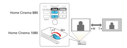
To sharpen the image, turn the focus ring.
