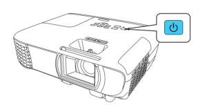
**Note:** To shut down the projector, press the **b** power button twice.
