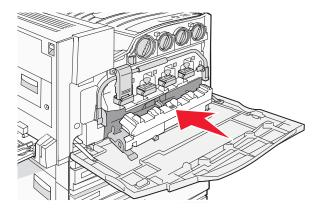
**9** Place the printhead lens cleaner in the notches of Door E.
