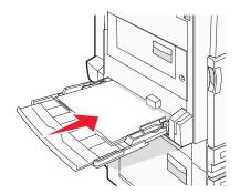
Load A3, A5, B4, folio, legal, and statement paper with the recommended print side facedown and the short edge of the paper entering the printer first.
