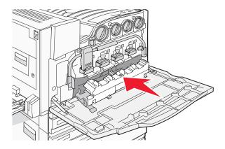
10 Place the new printhead lens cleaner in the notches of Door E.
