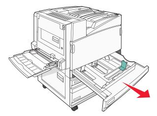
2 Squeeze the width guide tabs together as shown, and move the width guide to the correct position for the paper size being loaded.
