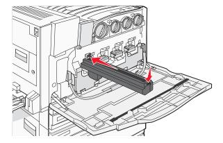
**8** Lift the bar up, and then press latch E5 down so that it holds the bar in position.
