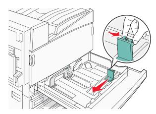
**3** Squeeze the length guide tab inward as shown, and slide the guide to the correct position for the paper size being loaded.
