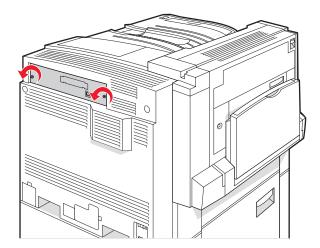
**b** Gently pull the cover and system board away from the printer, and then remove it.
