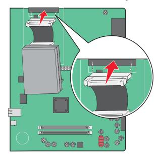
**6** Flip the hard disk over, and then press the three posts on the mounting plate into the holes on the system board. The hard disk *snaps* into place.
