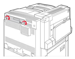
3 Tighten the screws firmly.
