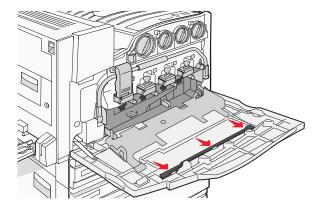
5 Insert the padded tip of the printhead lens cleaner into the first printhead lens opening.
