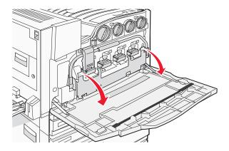
4 Remove the old printhead lens cleaner from Door E, and then discard it.
