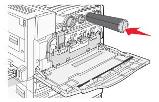
7 Lock the cartridge by turning the arrow-shaped cartridge handle clockwise until it points toward the lock symbol.
