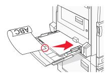
**Note:** Place the letterhead facedown in the multipurpose feeder with the long edge of the paper entering the printer first.
