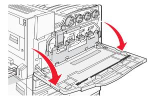
Unlock the specified cartridge by turning the cartridge counterclockwise until the arrow-shaped handle points toward the unlock symbol.
