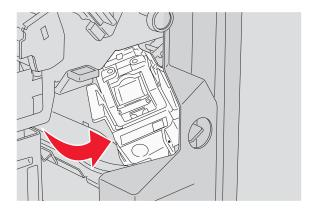
**3** Lift the lever, and then remove the staple cartridge.
