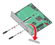
4 Align the connector on the internal print server or port interface card with the connector on the system board.
