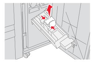
**9** Remove the jammed staples, and then place the staple cartridge into the stapler.
