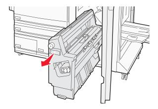
7 Lift the inside cover. If the paper is jammed in the rollers, rotate Knob G8 clockwise, and then remove the jammed paper.
