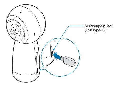
2 After fully charging, disconnect the Gear 360 from the charger. First unplug the charger from the Gear 360, and then unplug it from the electric socket.
