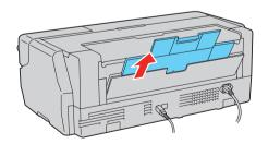
**2** Press the front cover to open it, if necessary, then fully extend the output tray.
