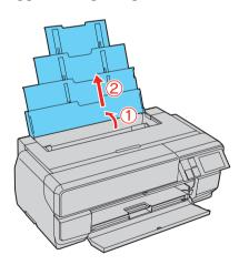
3 Insert paper, glossy or printable side up, short edge first, against the right side and beneath the tab. Then press the button on the edge guide and slide it against the paper.
