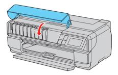
5 The printer begins charging the ink delivery system. This takes about 10 minutes. Do not turn off the printer, load paper, or open any covers until the process is complete.
