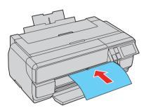
6 Feed the paper up to the line on the tray. Make sure the paper is flush against the right, then pull the paper back gently to align it against the edge of the manual feed tray.
