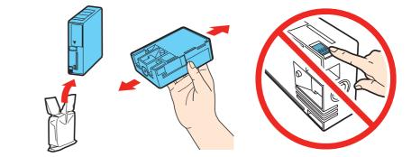
**3** Insert the cartridges in the slot for each color. Push the cartridges in until they click.
