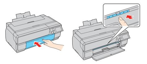
5 Insert a single sheet of fine art media. Insert it short end first with the printable side faceup.
