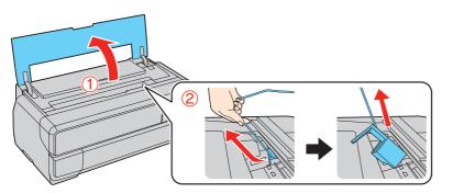
4 Press the front cover to open it and remove the transportation lock.
