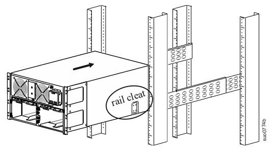
• Secure the UPS to the rack. Use four screws in each bracket. **5** Install four battery modules.
