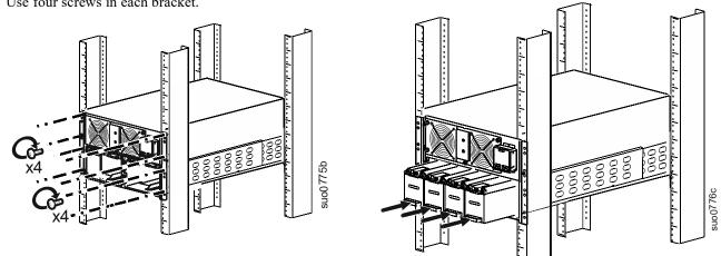
• After the UPS is hardwired to branch circuit mains complete steps 6-8. Connect all four battery modules.
