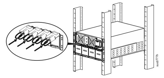
Reinstall the battery compartment doors.
