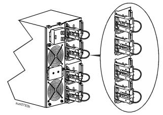
Reinstall the battery compartment doors. Tighten the thumbscrews to secure the doors.
