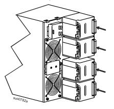
After the UPS is hardwired to branch circuit mains, complete steps 2-5.Connect all four battery modules.
