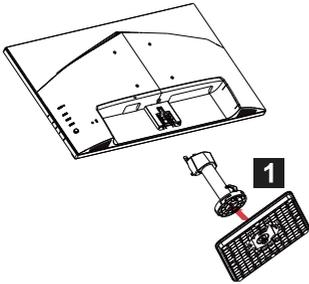
2. Ensure that the Lock alignment mark on the bottom of the base is aligned with the stand arm.
