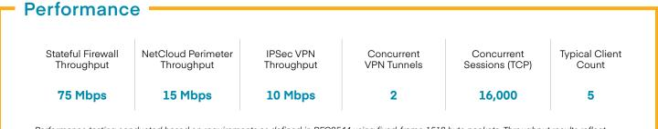
Performance testing conducted based on requirements as defined in RFC2544 using fixed-frame 1518 byte packets. Throughput results reflect uni-directional UDP traffic with less than 1% packet loss as tested with wired connections.
