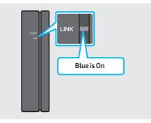
The LINK LED indicator stops blinking and glows a solid blue when a connection is established between the Soundbar and the Wireless Receiver Module.
