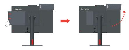
3. Press the computer from the front until it completely snaps into position.
