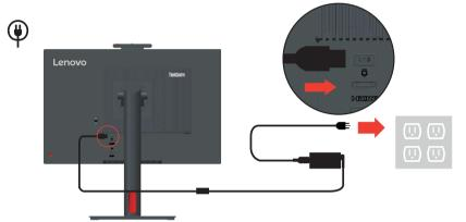
**Note:** When installing the computer to the TIO monitor for AIO mode, ensure you use the power adapter that comes with the computer when computer power adapter large than 90W, otherwise please use TIO power adapter.
