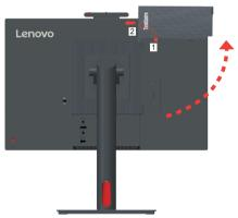
2. Screw the rear Wi-Fi antenna to the antenna connector on the rear of the computer. Then, adjust the angle of the antenna to 90 degrees.
