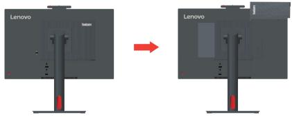
3. Pull the computer out of the computer bay. Then, pivot the cable cover as shown to the closed position.
