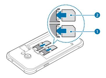
► Single SIM models: Insert the SIM or USIM card with the gold-coloured contacts facing downwards.
