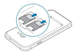
► Single SIM models: Pull out the SIM or USIM card.
