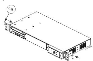
**3** Two-post rack-mounting: Utilize the bracket holes that are offset 6.25".
