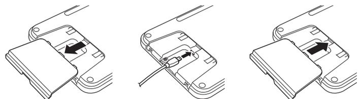
2. Connect the USB cable on the keyboard LCD unit to the socket on the side of the machine.
