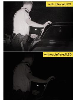
Infrared LEDs for low light conditions and night vision
