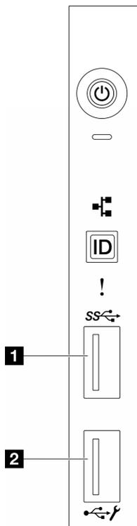
Figure 1. Connectors on the front I/O module
