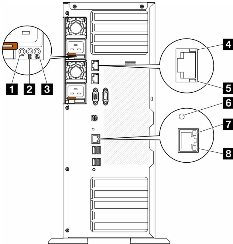
Figure 12. Rear system LEDs of the server
