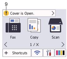
The warning icon papears when there is an error or maintenance message; press to view the details, and then press to return to the Home screen.
