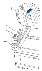
6. If your LCD displays [Jam Manual Feed Slot] or [Repeat Jam Manual Feed Slot], slowly pull the jammed paper out of the manual feed slot.
