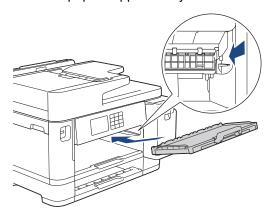
9. Replace the tray top cover and slowly push the paper tray completely into the machine.
