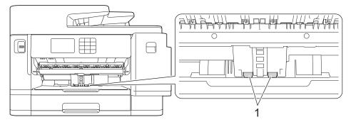
6. Place the paper support firmly back in the machine. Make sure you fit the paper support into the channels.
