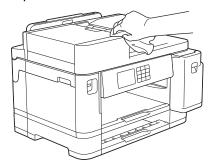
5. Remove the tray top cover and remove anything that is stuck inside the paper tray.
