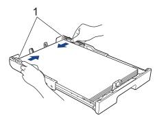
10. Make sure the paper is flat in the tray and below the maximum paper mark (1). Overfilling the paper tray may cause paper jams.
