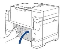
5. If your LCD displays [Jam MP Tray] or [Repeat Jam MP Tray], push the release lever (1) toward the back of the machine, and then slowly pull the jammed paper out of the MP tray.
