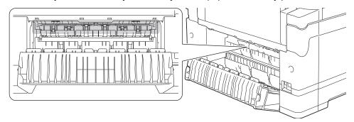
c. Close the Jam Clear Cover. Make sure the cover is closed completely.
