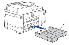
3. Lift the paper support (1), and then pull it at an angle completely out of the machine as shown by the arrow.
