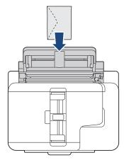
When loading an envelope, or a sheet of thick paper, push the envelope into the manual feed slot until
