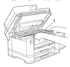
If your LCD displays repeat paper jam messages, for example [Repeat Jam Rear], move the print head, and then remove any paper remaining in this area. Make sure pieces of paper are not left in the corners of the machine (1) and (2).
