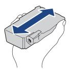
4. Insert the ink cartridge in the direction of the arrow on the label. Each color has its own correct position.
