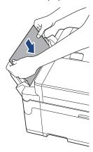
4. (MFC-J5855DW/MFC-J5955DW) Follow the instructions on the LCD to locate and remove the jammed paper.
