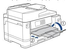
2. Pull the paper tray completely out of the machine as shown by the arrow.
