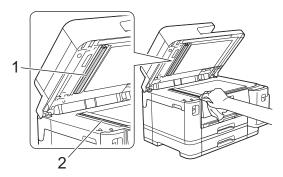
4. (MFC-J5955DW) Open the scanner glass cover (1), and clean the white bar (2) and the glass strip (3) with a soft lint-free cloth moistened with water.
